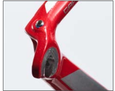
Figure 12. Threaded hole in left rear dropout
